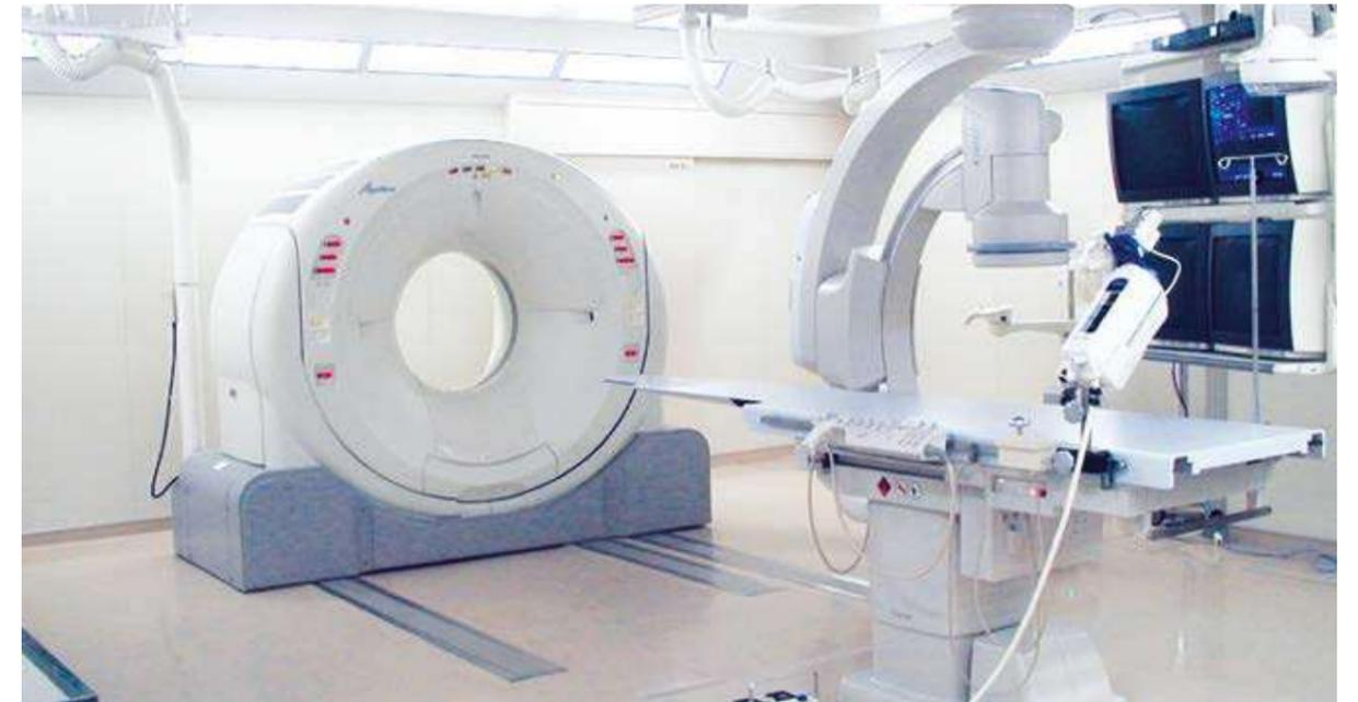
Figure 7: The ceiling C-arm can park perpendicular to the table and CT gantry. This unique design doesn't disturb patient approach from both right and left side of the patient
