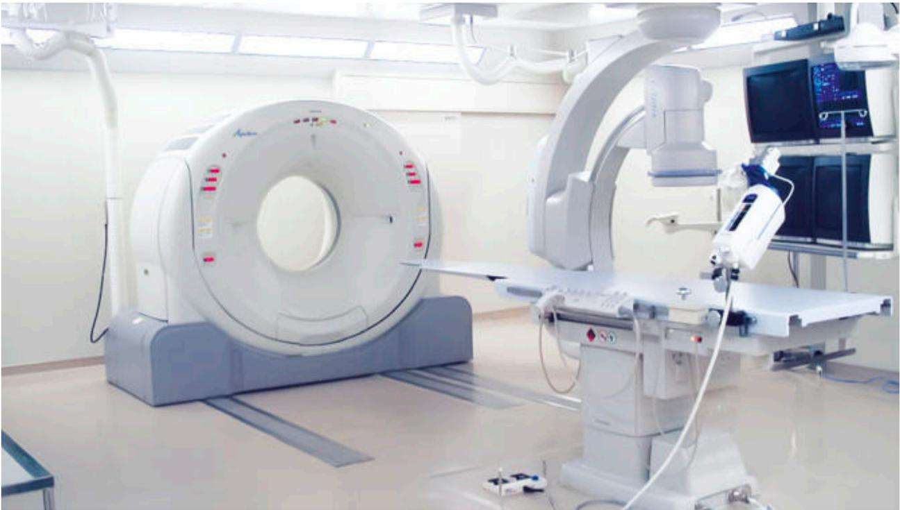
Figure 7: The ceiling C-arm can park perpendicular to the table and CT gantry.
