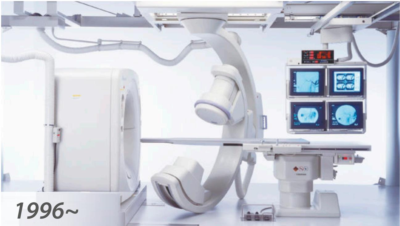
figure 5: The Angio CT system produced in 1996. The CT gantry is now movable on the floor rail.
