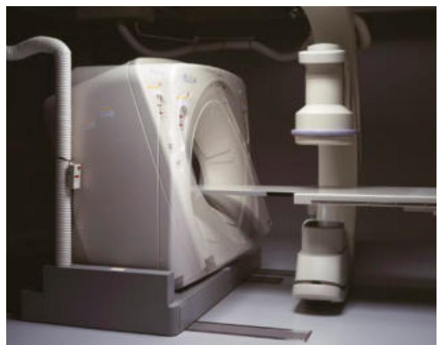
The CT base can move on the floor to realize the helical scan. This unique concept was born by Toshiba/Canon in 1996.
